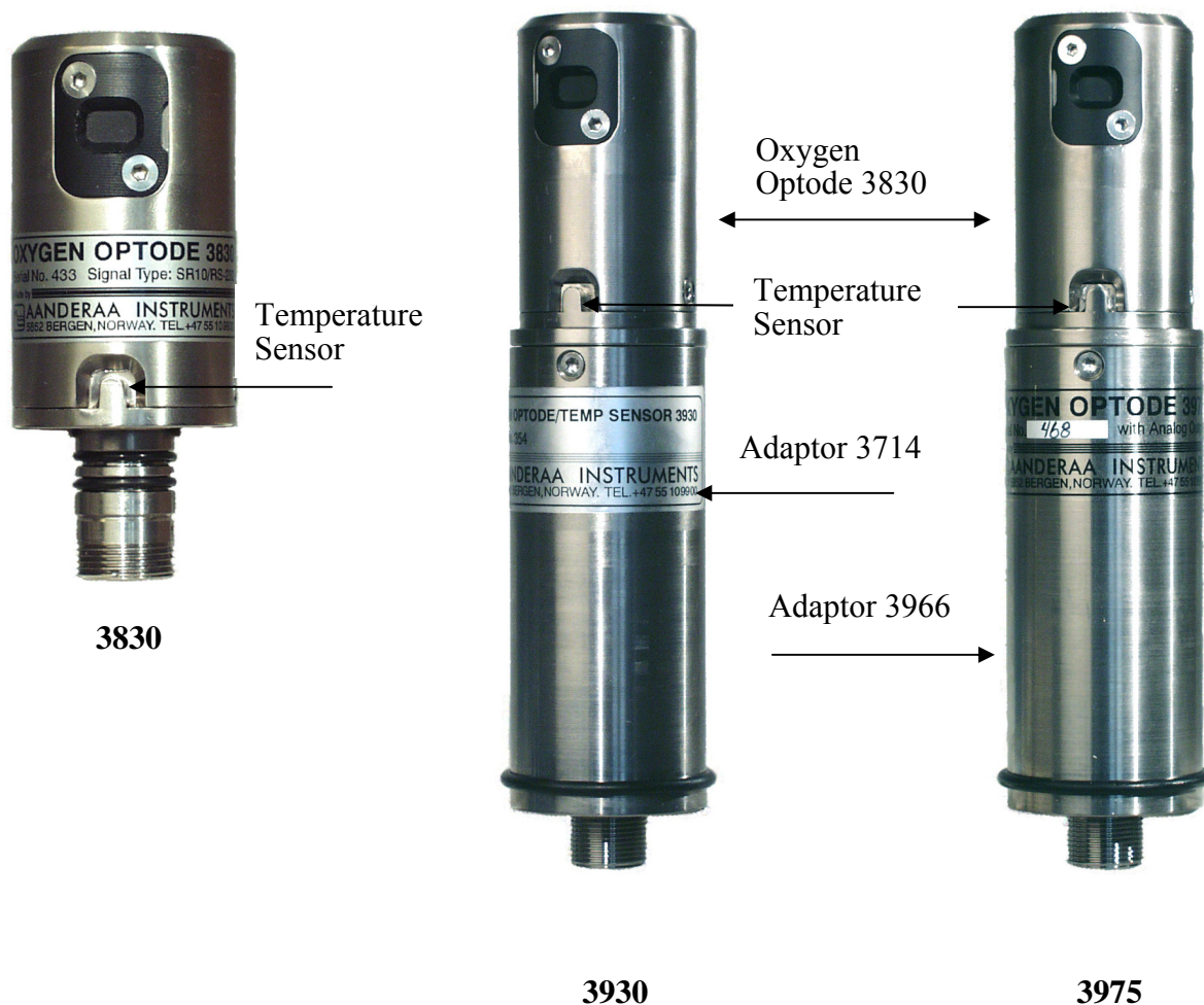
Figure 1 Illustration of the Oxygen Optode 3830 (to the left), 3930 (in the middle), and the 3975 (to the right)
