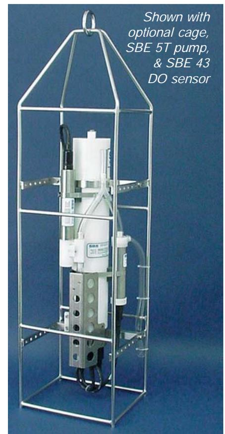
*Shown with optional cage, SBE 5T pump, & SBE 43 DO sensor*
