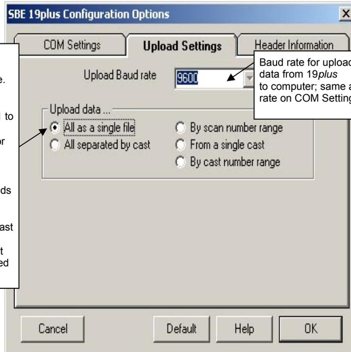
Baud rate for uploading data from 19plus to computer; same as baud rate on COM Settings tab.
