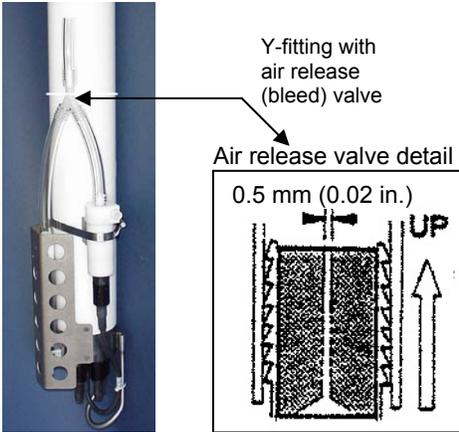
For SBE 19*plus* with plumbing configured for vertical orientation - Periodically clean the air release valve with a 0.4 mm (0.016 inches) diameter wire (you can use #26 AWG wire), and blow through it to ensure it is open. **A clogged air release valve can trap air, preventing the pump from functioning properly;** this will affect the data quality.
