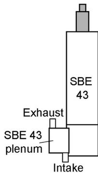
Place DO sensor with plenum intake closer than exhaust to SBE 43 housing as shown.
