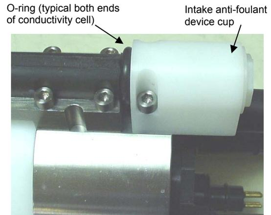
5. Check the exhaust end of the conductivity cell to ensure that the o-ring is still in place.
