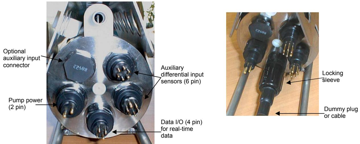
2. Connect the other end of the cables installed in Step 1 to the appropriate sensors.
