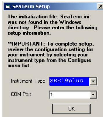
Select the instrument type (*SBE 19plus*) and the computer COM port for communication with the 19plus. Click OK.
