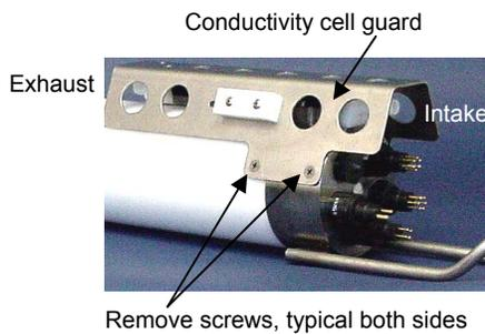
2. Remove the four Phillips-head screws attaching the conductivity cell guard to the housing and end cap. Carefully remove the conductivity cell guard.
