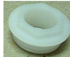
Note: The larger diameter of the intake cap / non-pumped application exhaust cap helps maintain good flow through the conductivity cell and reduces growth of biological material. **Do not use the barbed cap in its place.**
