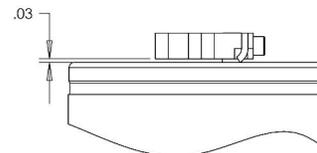
12. Use the 3/32-in. hex key to tighten the screw to "finger-tight," then snug an additional quarter-turn.
