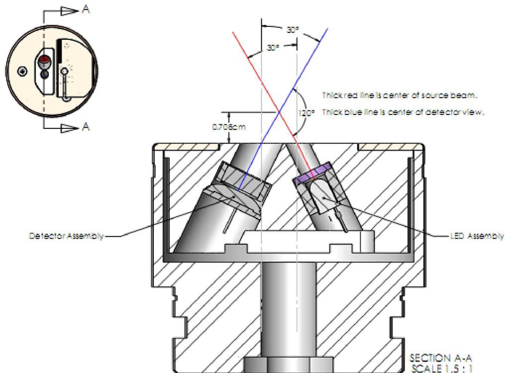
**Optical configuration of *ECO* scattering meter**
