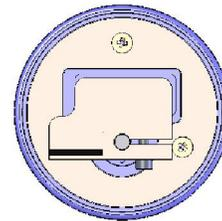
11. Set the gap between the *Bio-wiper*<sup>™</sup> and the instrument face to 0.03 in. (0.8 mm). An improperly set gap will either fail to clean the face or cause the motor to draw excessive current.
